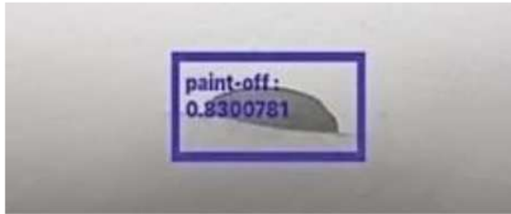
Figure 4: Real-time visual detection of aircraft skin defects (paint-off class) using YOLO11 deployed natively on mobile edge devices.
